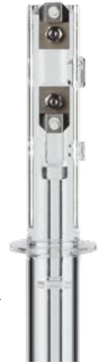
Tensile test of a polycarbonate film between -10°C and 190°C
